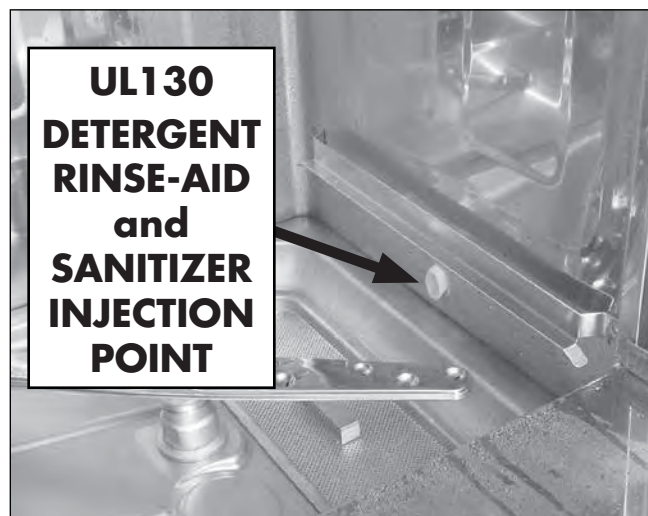
On the UL130, chemicals enter the wash tank through a fitting on the right-hand side of the tank.
