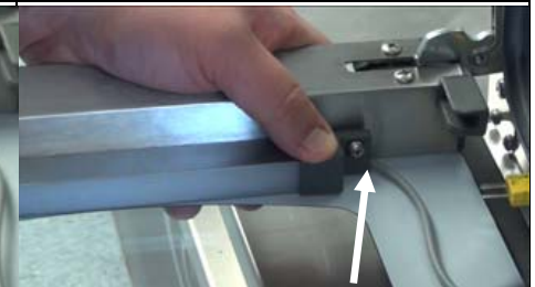
Fig. R 13) Attach the bottom cover bracket, making sure the wire is seated in the wire notch.
