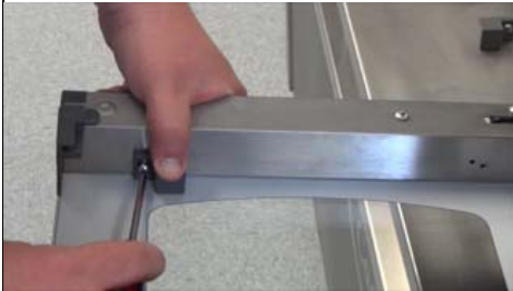
Fig. M 9) Replace the top cover bracket, but do not fully tighten the screws yet.
